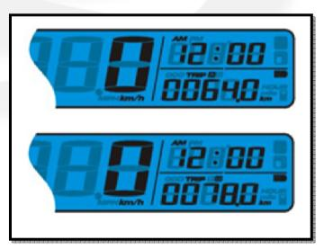
**TOTAL HOUR:** Press the **Adjust button** to switch from trip B to total hour meter.
