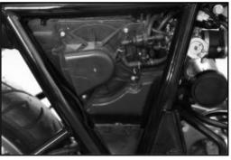
■ Remove airfilter element from the housing.
