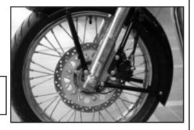
Flanged Hex bolt: M8 Socket Spanner: 12 mm
