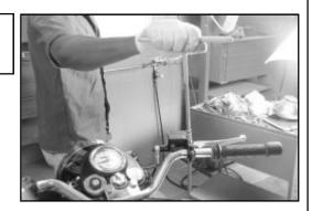
■ Remove master cylinder assembly from the handle bar and support suitably to prevent hydraulic oil leak from master cylinder.
