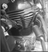
It senses the oil temperature and provides the input to the ECU on a real time basis. The ECU can then determine the fuel injector operating time to provide the required amount of vaporized fuel into the combustion chamber for optimum performance of the motorcycle and also to meet the emission norms.
