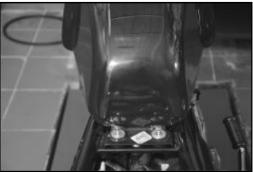
**Hex Flange Bolt M6 Socket Spanner 10 mm** Torque 5 Nm
