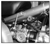
It consists of a throttle plate (butterfly valve) to regulate the airflow into the cylinder head depending on the throttle opening and a manual Bi Starter which helps control idling RPM in extreme cold conditions.
