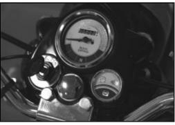
When both the Ignition & Engine kill switch is "ON" and after vehicle is started, MIL will glow for few seconds and switch in the Ignition of IgnitiOFF, this indicates that all the functions of EMS are functioning correctly.
