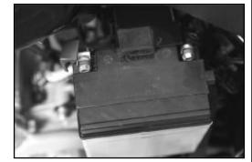
Pull the battery out slightly from the battery carrier.
