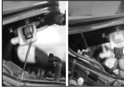
**Hex Flange Bolt M6 Socket Spanner 10 mm**
