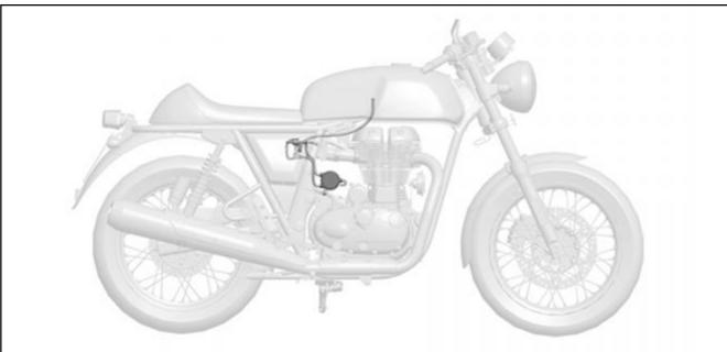
The system consists of a canister, purge valve, rubber hoses, connectors and a sealed fuel tank cap.
