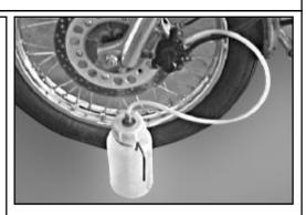
with 'Fresh brake fluid' from a sealed container till "MAX" level.
