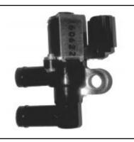
In addition to the Hego sensor, the EXAI gets inputs from the ECU to supply filtered air into the exhaust end of the cylinder head, primarily during idling RPM so as to meet exhaust emission specifications.
