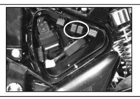
The EFI ECU Power relay supports functioning of the ECU and fuel pump. The Side stand relay provides the inputs regarding the position of the side stand to the ECU. In the event the side stand is NOT retracted and the motorcycle is attempted to be started, it signals the ECU which cuts off the fuel supply thus preventing the engine from starting.
