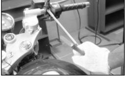
■ Remove the 2 rubber **Hex. Socket Head Screw:** grommets on top of the **M8** handle bar LH & RH and remove the 2 hex socket Allen Key: 6 mm head cap screws.
